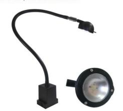
6W LED lamp made up of aluminum and ABS illuminator, stainless-steel gooseneck arm covered by a PVC sheath, ABS base with fastening holes, on/ off switch and built-in LED driver.
